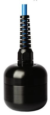
The OxyGuard Probe is a membrane covered galvanic cell that generates an electrical signal proportional to the oxygen pressure it senses, no matter whether it is in water, air, gas, wine, oil or something else. The probe can be used to measure dissolved oxygen in aquaculture, the environment, in clean water, waste water and in oil or other fluid. It can measure very small oxygen concentrations in inert or explosive gases as well as the oxygen content of ambient air and the purity of oxygen gas.
